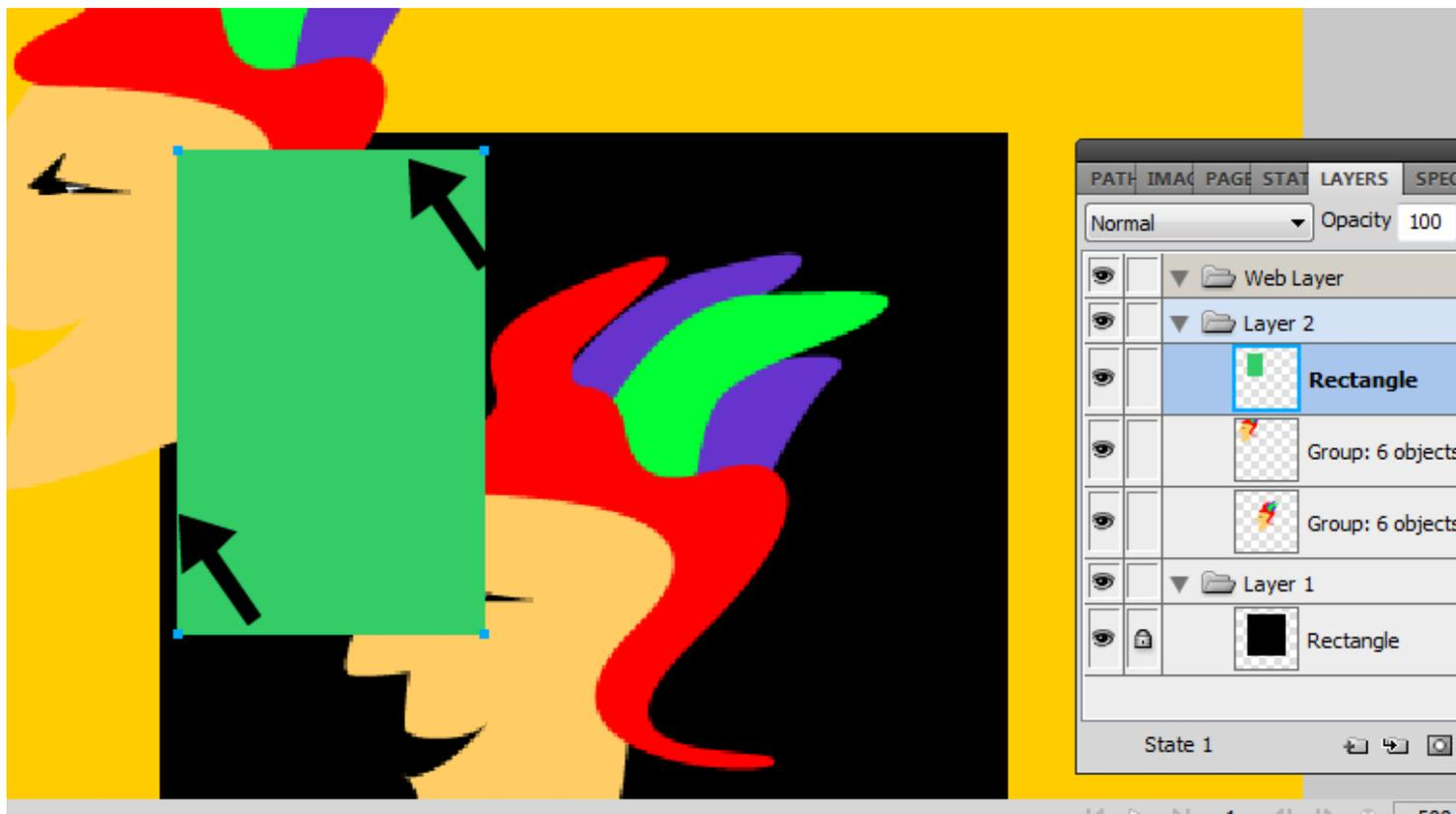
Duplicate the corner set including the colored rectangle and slide over to right, being careful to match top edge of colored rectangle with the inside edge of the underlying rectangle. Slide over until the colored rectangle no longer overlaps the underlying rectangle.
